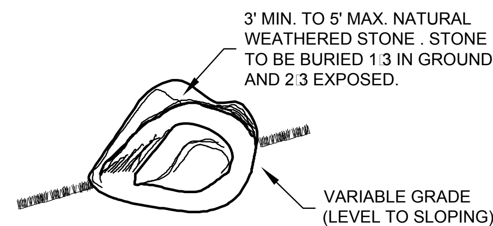
BOULDER PLACEMENT DETAIL TYPICAL
